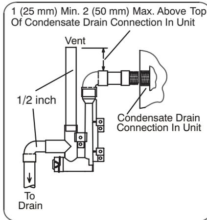
Drain Trap Assembly with 3/4 inch Piping
