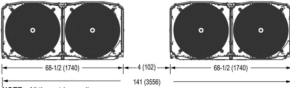
**NOTE - All the outdoor units manifolded together should be installed at the same elevation.**
