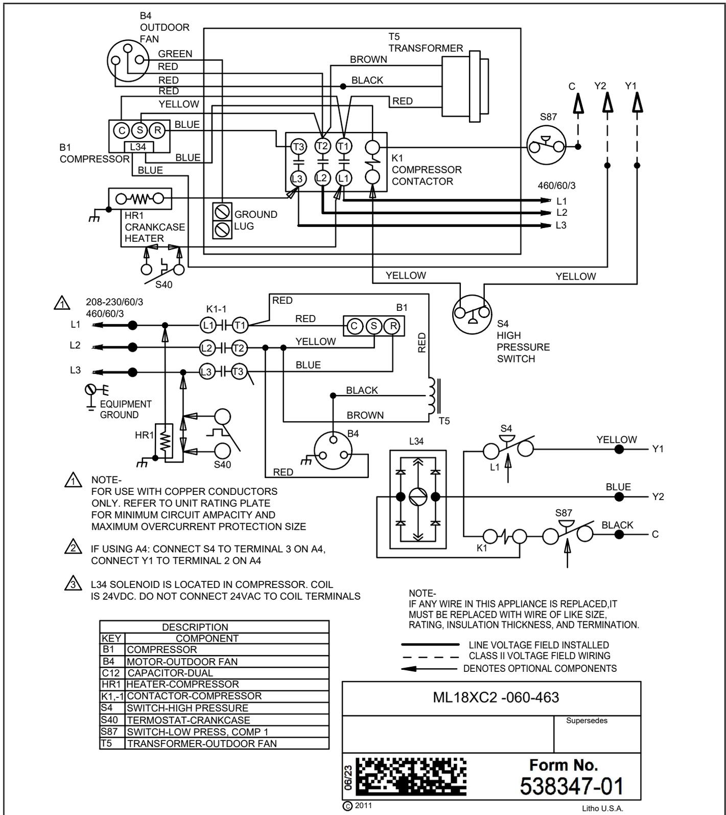
FIGURE 13. Typical Wiring Diagram -- -060 (G Voltage)
