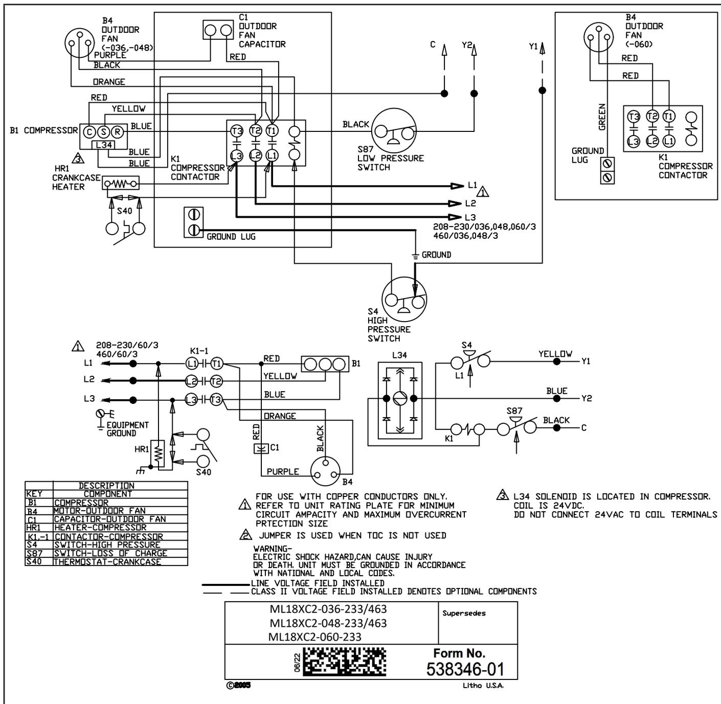
FIGURE 12. Typical Wiring Diagram – -036, -048 (Y and G Voltage) and -060 (U Voltage)
