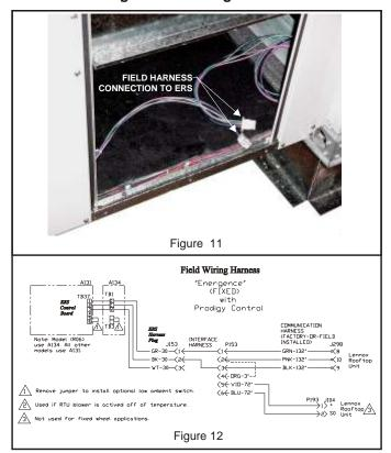
11. All electrical connections must conform to any local codes and the current National Electric Codes (NEC) and Canadian Electric Code (CEC). Refer closely to wiring diagram in unit and/or in these instructions for proper connections. Refer to the unit nameplate for the minimum circuit ampacity and maximum over current protection size. Electrical data is listed on unit rating plate and motor nameplates.
