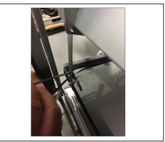
Figure 12. Relocate T-1 Sensor
