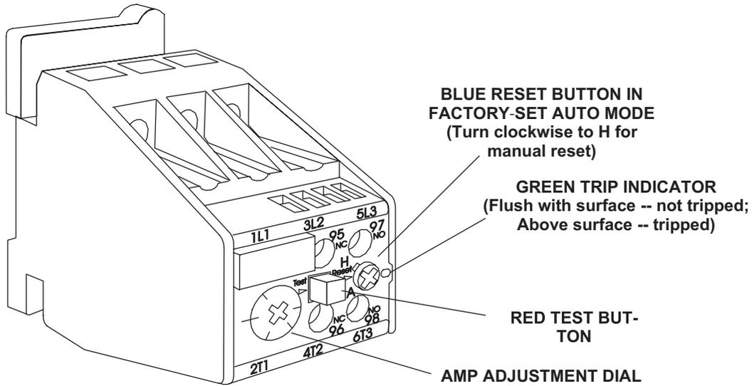
Adjust relay amp setting according to value given on the blower motor nameplate. Proper relay amp setting equals motor nameplate FLA X service factor of 1.15 X .95.
