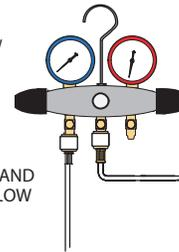
**F** CONNECT GAUGES AND START NITROGEN FLOW
