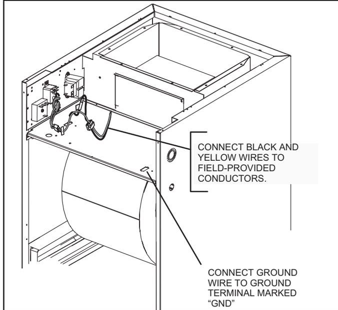
**FIGURE 23. Making Electrical Connections**
